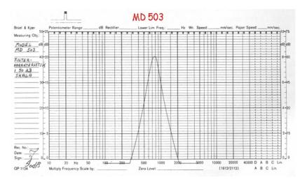
Filter curve from the original 'BSP MD503 CW filter' (1978), of which the MD6 CW-AF is a 'modern' version.
