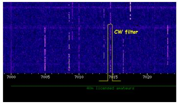
Typical CW signals on, for example, 40 meters and use of the filter.
